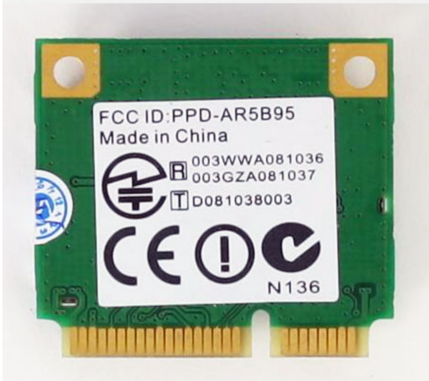
Wireless LAN Mini-PCI Express card Azurewave AW-NE785H Atheros AR9280 / AR5B95 chipset (802.11b/g/n)
